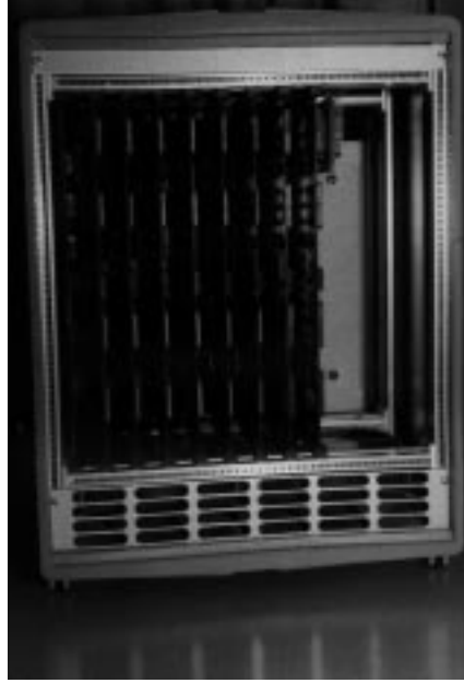
Figure 3: MIT Laboratory for Computer Science cellular automata machine CAM-8. This 8 module prototype can evolve a D-dimensional cellular space with 32 million sites where each site has 16 bits of data with a site update rate of 200 million per second.
