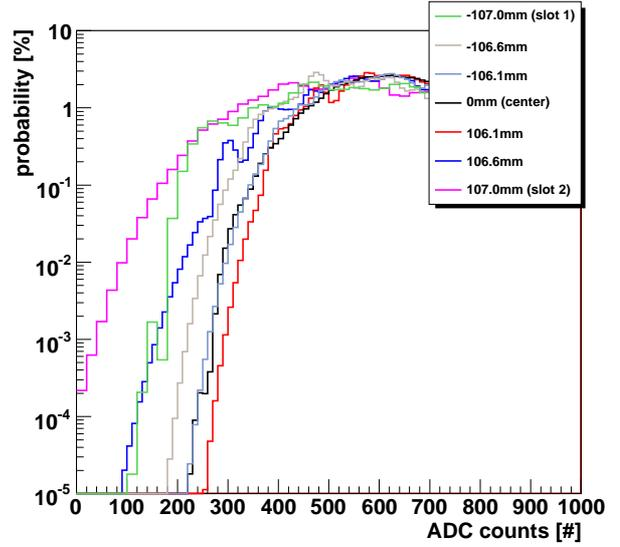
**Figure 4.162:** Normalized and smoothed pre-integration ADC spectra for the inefficiency calculation.
