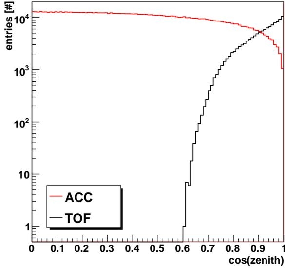
Figure 4.165: Zenith angle distribution of cosmic rays in TOF and ACC.
