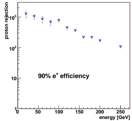
Figure 4.6: Proton rejection at 90% positron efficiency vs. proton energy<sup>[110]</sup>.
