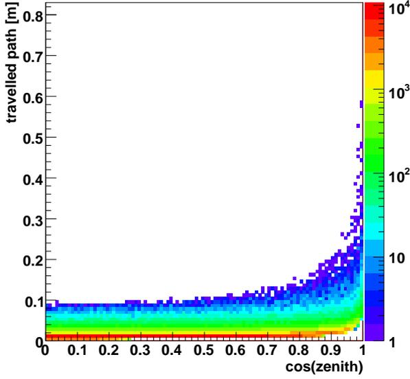
**Figure 4.159:** Pathlength travelled in the ACC as a function of the zenith angle. The color code on the right shows the number of entries.
