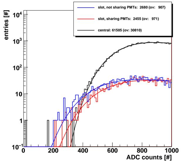
**Figure 4.149:** Highest ADC values of the complete ACC system for the central region of the ACC panels and the two different slot regions in an interval of 15 mrad around the slots. The vertical line indicates the cut for the definition of a good event.
