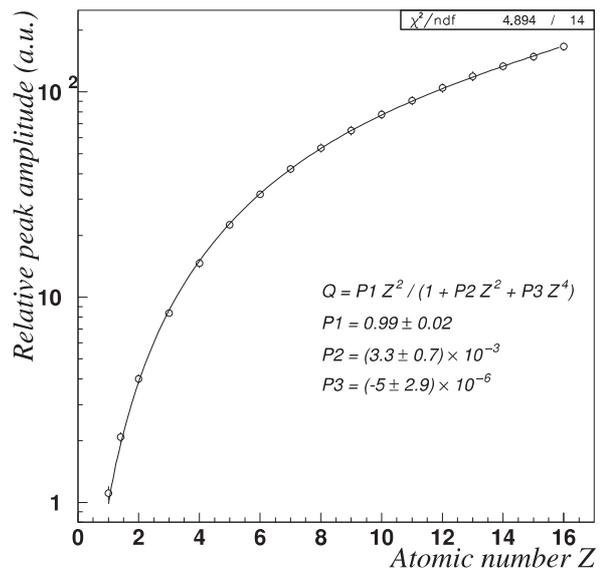
Figure 4.9: TOF: amplitude vs. charge<sup>[114]</sup>.
