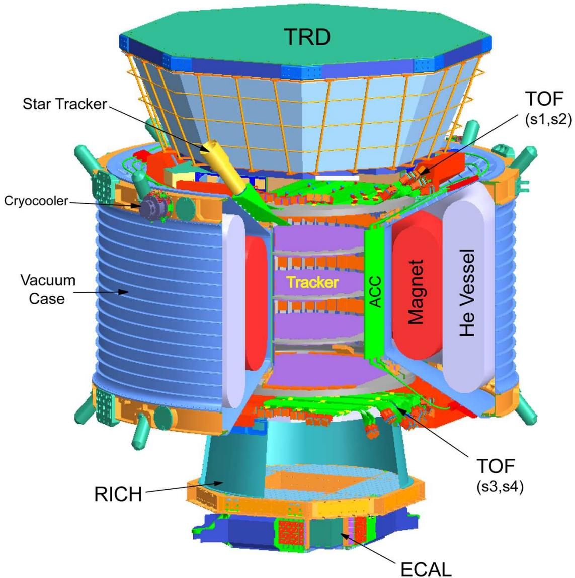
Figure 4.4: The AMS-02 experiment<sup>[112]</sup>.
