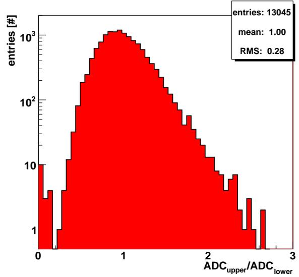
**Figure 4.154:** Signal ratio of upper and lower PMTs in the central region  $z = 0$  cm normalized to a mean of 1.
