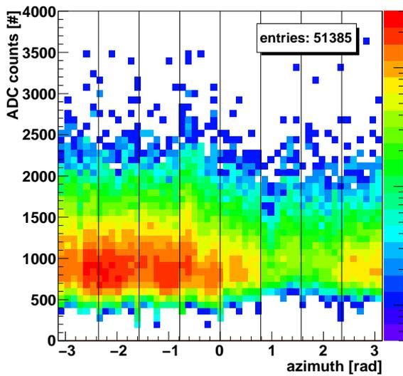
Figure 4.151: ADC values of the  $-z$  PMTs as a function of the azimuthal angle for the case that these PMTs have recorded the highest ADC value. The vertical lines indicate the slots between the ACC sectors. The color code on the right shows the number of entries.
