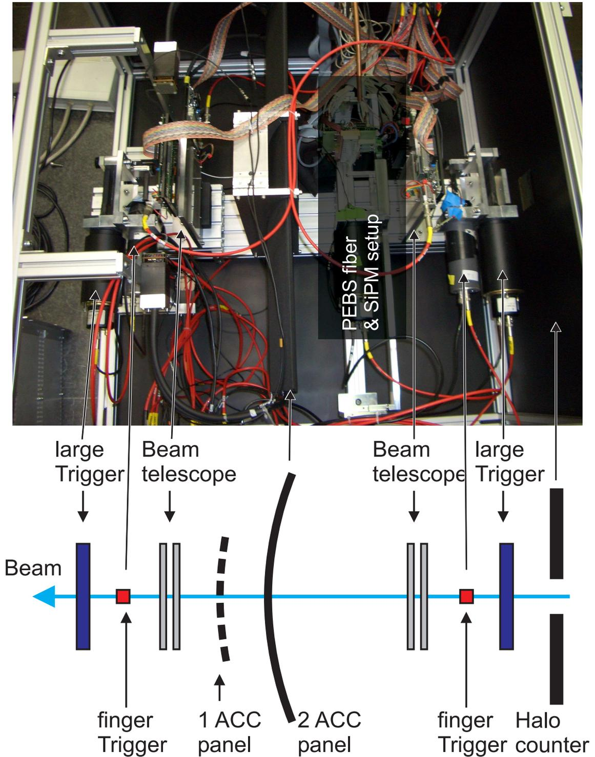
Figure 4.61: Testbeam setup.
