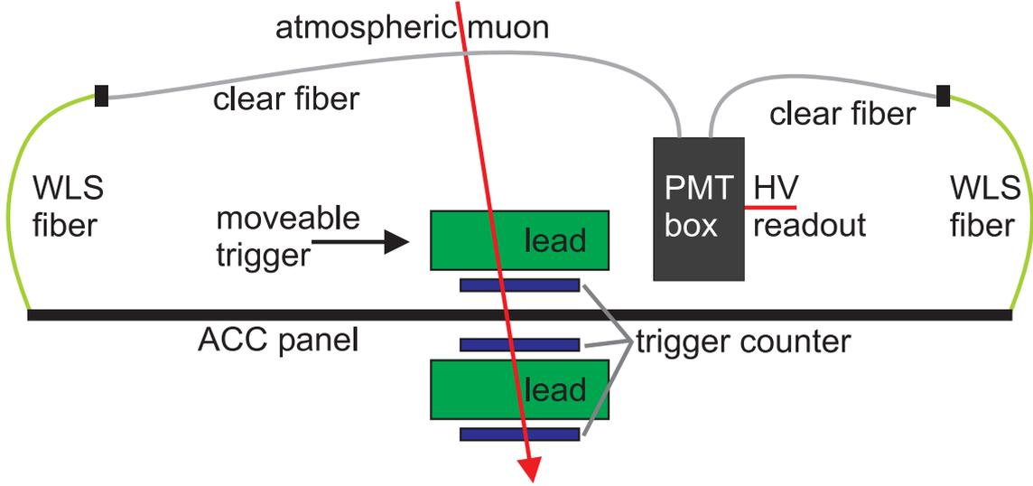
Figure 4.83: Setup for ACC performance tests.
