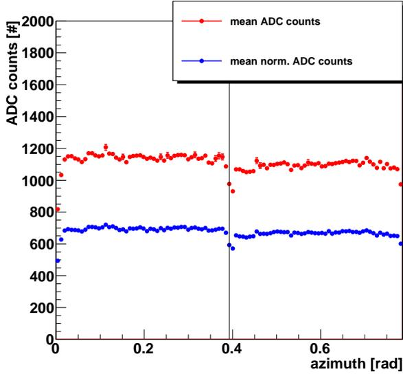
**Figure 4.157:** Mean (normalized) ADC values vs. the azimuthal position in an ACC sector. The line indicates the slot between the two panels of the sector.
