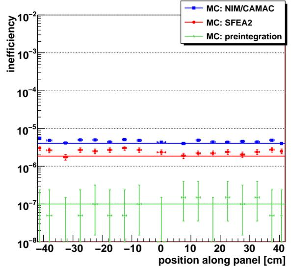
**Figure 4.164:** Expected inefficiencies along an ACC panel. The horizontal lines indicate the corresponding mean values.
