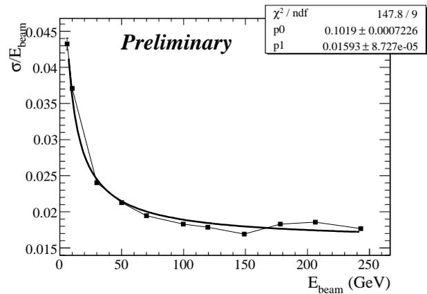
Figure 4.14: Energy resolution of ECAL<sup>[117]</sup>.
