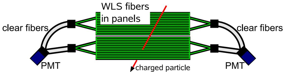
Figure 4.26: ACC principle.
