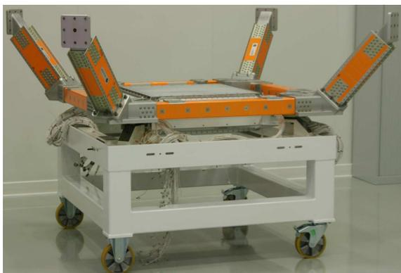
Figure 4.13: Electromagnetic calorimeter in the AMS-02 clean room.
