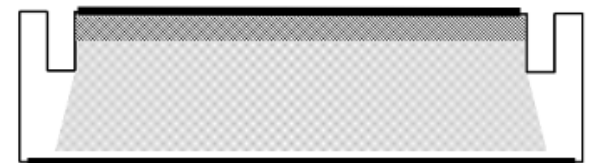
(c) Drift Li through wafer
