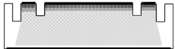
(e) Cut guard ring groove and re-apply contacts
