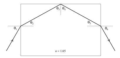
**b.** (5 pts.) Calculate the **critical angle** between the prism and air. Show your work! Relatedly, briefly **explain** what happens when the ray hits the top side of the prism, resulting in  $\theta_3$  and  $\theta_4$ ... what is this phenomenon called?
