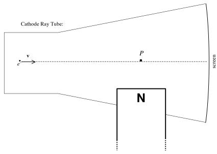
**d.** (4 pts.) Suppose that the electron momentarily passes through point P, where B = 0.0032 T, the electron's velocity is  $8.8 \times 10^6$  m/s, and the angle between **v** and **B** is exactly 90°. Calculate the **radius of curvature** of the electron's path at that instant.
