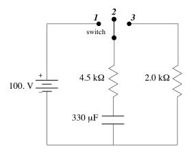
**b.** (1 pt.) What is the **potential difference across the capacitor** after the switch has been in position (1) for a very long period of time? (You do NOT need to show your work.)
