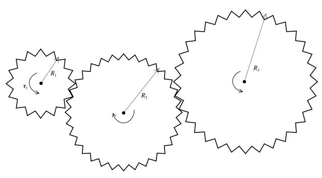
4. Three interlocking gears have average radii of  $R_1$ ,  $R_2$  and  $R_3$ , with relative sizes as shown above. (Their centers are all fixed, and there is no friction at their pivots. Assume that the size of the gears' teeth is much smaller than the gears' radii.)
