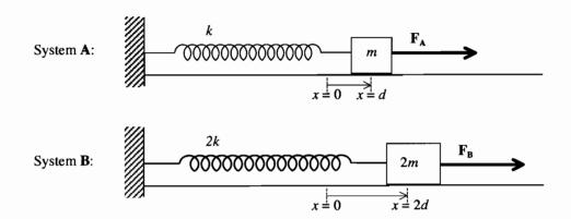
Questions #12-16: Masses m and 2m are attached to ideal, massless springs, k and 2k, respectively, as shown above. The mass in system A is initially pulled aside to a displacement of x = d, while the mass in system B is initially displaced twice as far. (The surfaces are frictionless. The force vectors  $F_A$  and  $F_B$  are NOT necessarily drawn to scale.)
