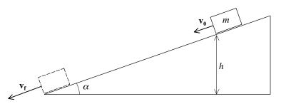
A mass *m* starts with an initial downhill speed  $v_0$  at height *h*, and slides down a *frictionless* incline of angle  $\alpha$ , as shown above.
