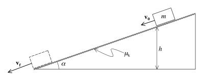
Suppose now that there *does* exist **kinetic friction**  $\mu_k$  between the mass and the incline, but all other initial conditions are unchanged. (Let the kinetic friction be fairly weak, so that the mass does reach the bottom of the incline, and does so with a final speed  $v_f > v_0$ .)
