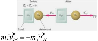
$\vec{v}_{Af} = -\frac{m_P}{m_A}\vec{v}_{Pf} = -\frac{(80 \text{ kg})}{(60 \text{ kg})}(-0.30 \text{ m/s})\hat{x} = (0.40 \text{ m/s})\hat{x}$
