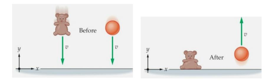
Change in momentum:  $\Delta p = p_{after} - p_{before}$ Teddy Bear:  $\Delta p = 0 - (-mv) = mv$ Bouncing Ball:  $\Delta p = mv - (-mv) = 2mv$
