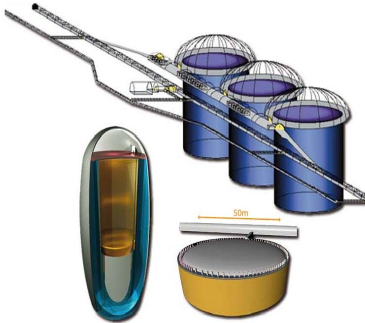
**Figure 1** Cartoons of the three large underground neutrino detectors under consideration in the European LAGUNA project, MEMPHYS (700 kT Water Cherenkov), LENA (50 kT liquid scintillator) and GLACIER (100 kT liquid argon).
