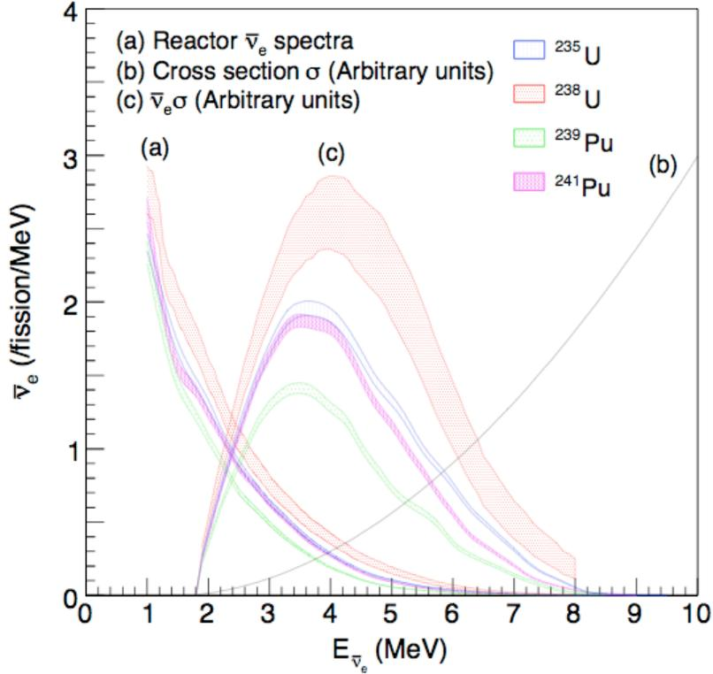
**Figure 2 Unoscillated reactor spectrum, including the contributions of various reactor materials (a), the inverse beta cross-section (b), and the event rate (c)**
