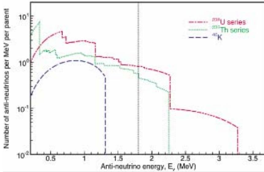
Figure 4 The expected  $^{238}\text{U}$ ,  $^{232}\text{Th}$  and  $^{40}\text{K}$  decay chain electron anti-neutrino energy distributions<sup>iii</sup>. The neutron-inverse-beta-decay detection reaction is only sensitive to electron anti-neutrinos to the right of the vertical dotted black line; hence it is insensitive to  $^{40}\text{K}$  electron anti-neutrinos.
