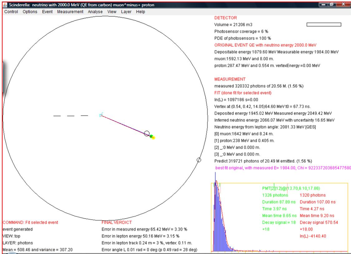
**Figure 11 Scinderella reconstruction of a 2 GeV quasi-elastic neutrino event in liquid scintillator. Note 3.15% resolution of neutrino energy, as well as short stub reconstructing recoil nucleon.**
