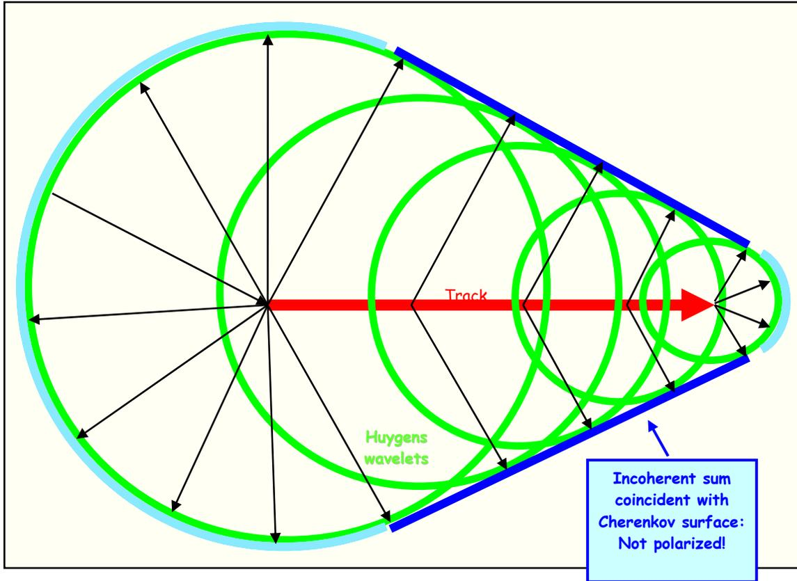
**Figure 10** Snapshot cartoon of the Fermat Surface from a single muon like track in liquid scintillator.
