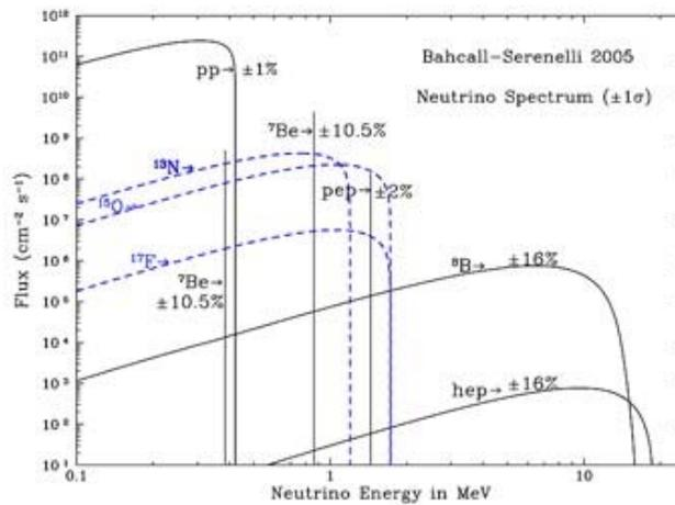
Figure 8 Neutrino energy spectra for the various reactions occurring in the Sun.<sup>vii</sup>
