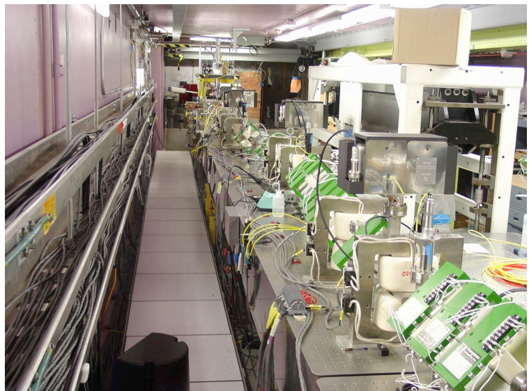
Figure 5. Diagnostic Chicane for Characterization of 6D eBeam Phase Space via Phase Space Tomography
