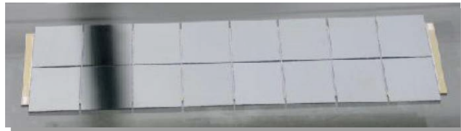
Diamond sensor ( \sim 2 \times 6 \text{ cm}^2 ) and 16 FE13 readout chips (Bonn)
