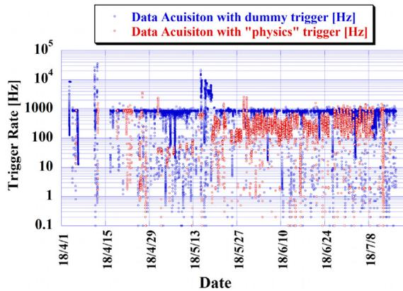
Fig. 3. History of trigger rates during the Phase2 run period. Here, “physics trigger” is for physics data-taking with beam collisions and “dummy trigger” is for DAQ test runs usually with a 1 kHz trigger with random time intervals. The DAQ test runs were done during accelerator studies with the high voltage of most detectors off.
