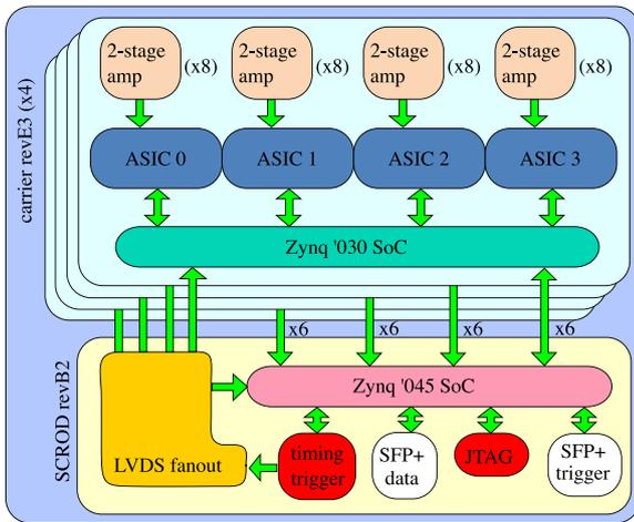
Fig. 1. Diagram of a TOP readout electronics module.
