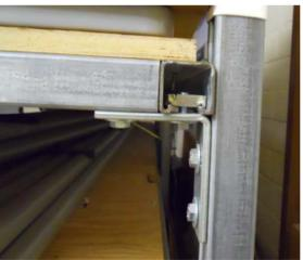
Center supports use large cantilever brackets. End supports use simple right angle brackets. The cantilever mid-supports allowed us to take the TOF counters in and out without moving other components.
