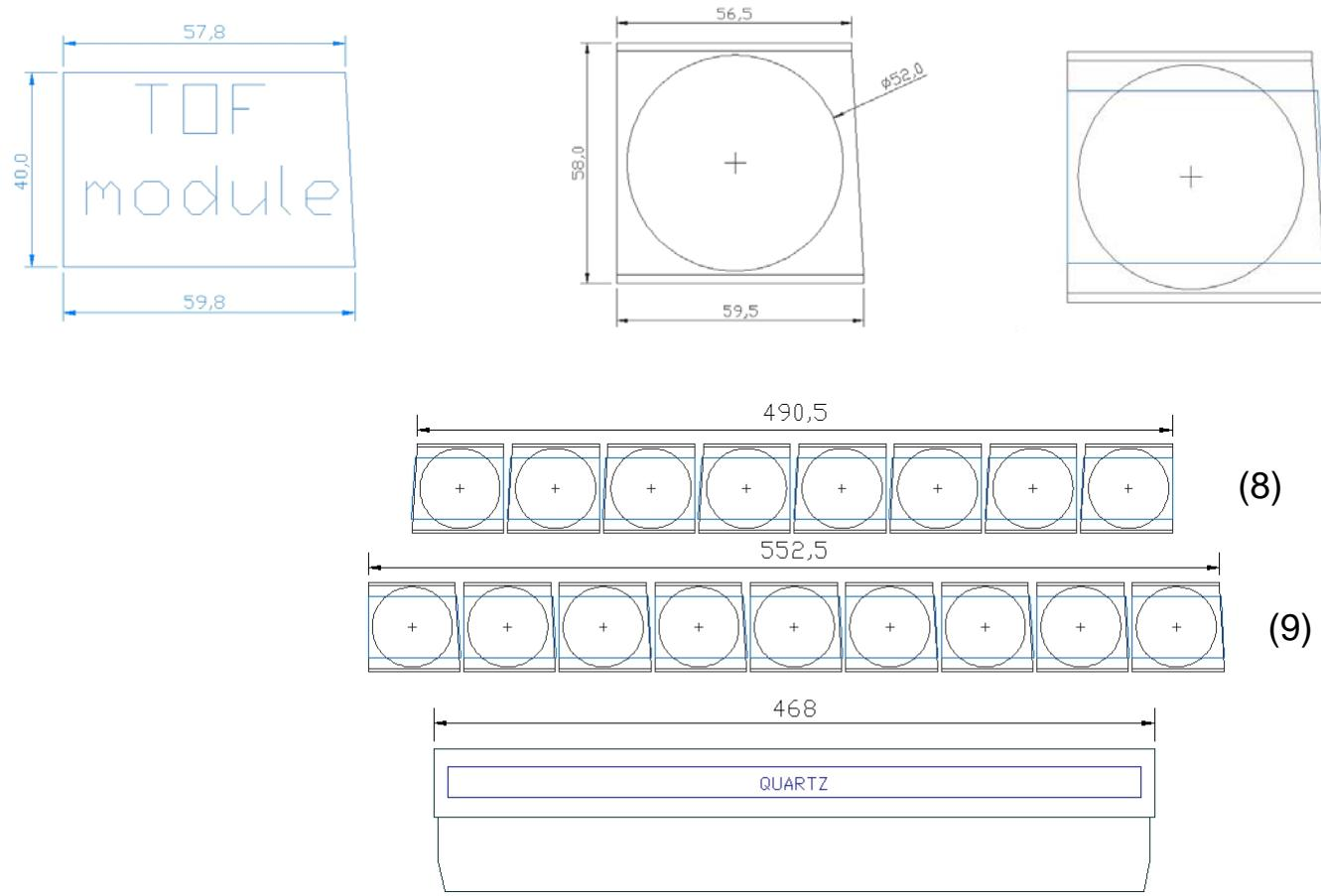
Eight TOF modules (min) are required to span one TOP module
