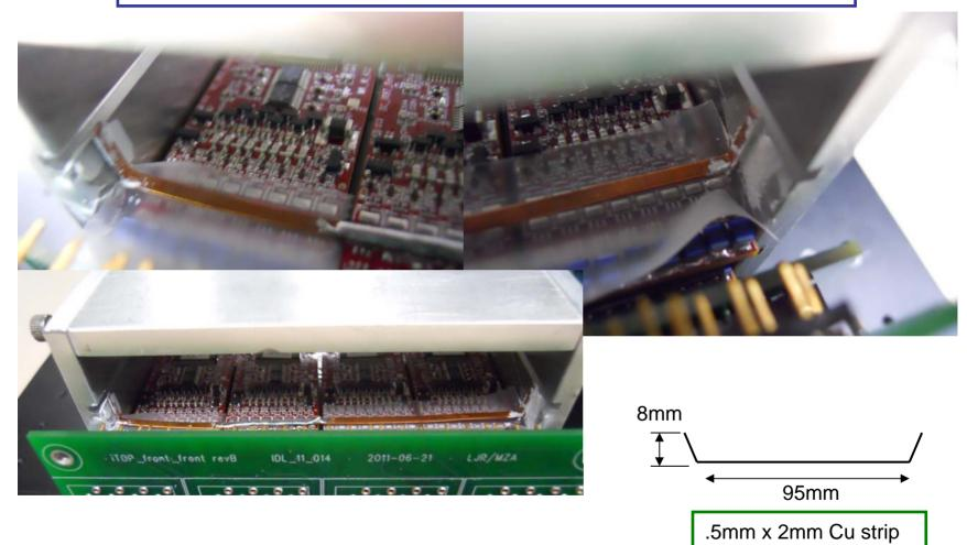
Thermal mitigation, step 2: mount the Nagoya Cu cooling plates to the upper and lower surfaces of the external housing.
