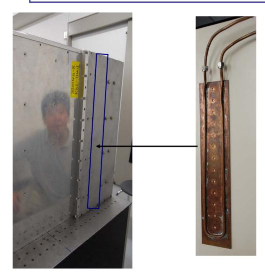
The Nagoya cooling plates will be cut down by 3-4mm and new threaded holes will be made in the in the large plates of the external electronics enclosure.
