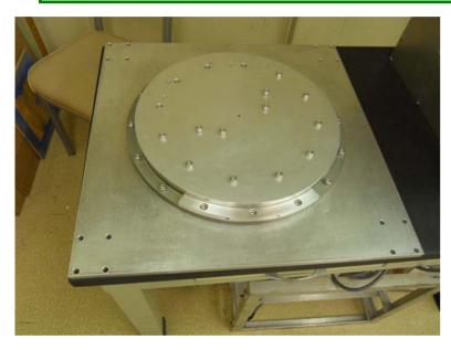
.5" thick base plate x 23.5" ^2, with 16" dia. rotating platform, ~50lbs.
