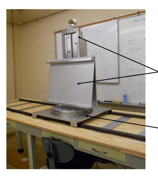
The vertical translation stage and the phi capture hardware are not compatible with the current beam test module due to size and mass considerations.
