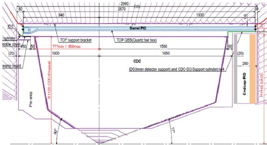
Figure 1: Cross-sectional view of the Belle II detector, where the restricted envelope available to the Barrel PID device is clearly seen.
