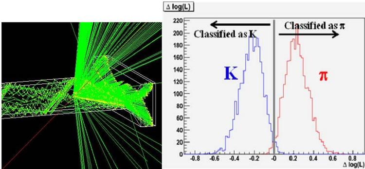
Figure 2: GEANT simulations (GEANT4 left) predict photon space-time Probability Density Functions to which photon data are compared to form a K/π Likelihood discriminator, as shown at right.
