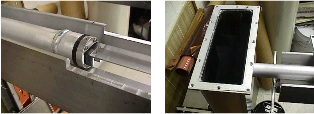
Fig. 6 – Photon trap at the end of 4 meter-long synthetic fused silica bar. The aluminum container, filled with a fused silica matching fluid, is coupled to a bar via a pipe equipped with a rubber seal. The aluminum container and pipe walls are covered with a photon absorbing cloth. The trap was very efficient eliminating the entire Cherenkov signal.
