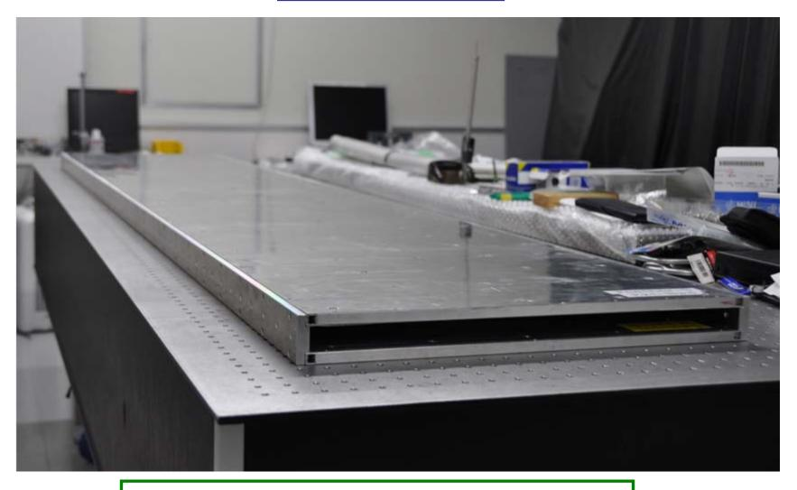
Side walls and honeycomb panels are 10mm thick.
