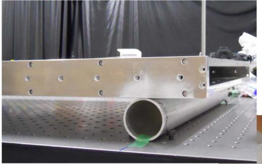
~42mm diameter aluminum pipe is secured to the optical table at each end of the QBB to allow for "simply supported" deflection measurements.
