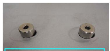
Shoulder screws in slots provide 4mm of travel in Z for optical coupling adjustment.
