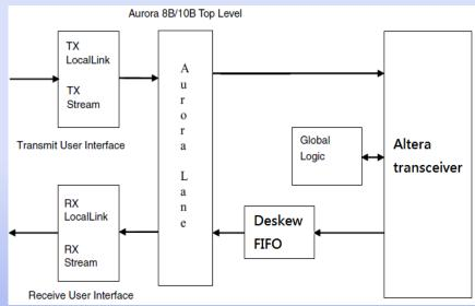
Figure 1-58. Deskew FIFO—Lane Skew at the Receiver Input
