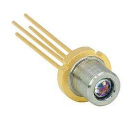
L1550P5DFB 1550 nm, 5 mW, Ø5.6 mm, D Pin Code DFB Laser Diode with Aspheric Lens Cap
