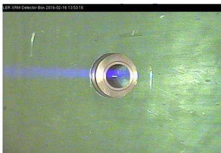
Figure 1.2 – The X-Ray entering the box through an orifice, side note: the picture has been taken without external light source...
