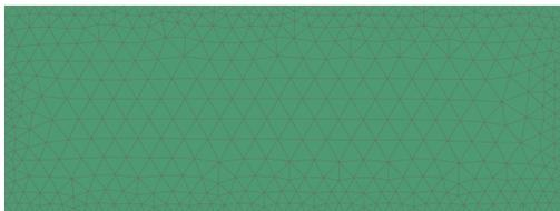
Epoxy layer, element size: 0.125 mm, 11005
