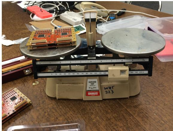
Figure 4.9 – Mass determination of 2 amplifier boards
