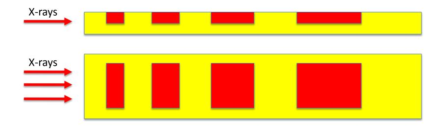
Beam enters on the side, not the front Strips are perpendicular to the beam Depth of interaction gives energy information Modest channel count (16?)
