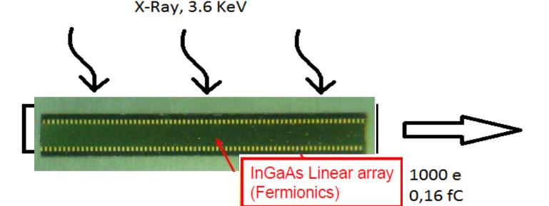
•The sensor response time is 0.5 nS, Signal low-high change time Δt is 0.25 nS.
