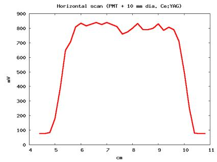
Horizontal width clipped: beam fills 5 cm of 8 cm window. Probably right edge (at 10 cm) corresponds to downstream window edge. Left edge due to upstream extraction window?
