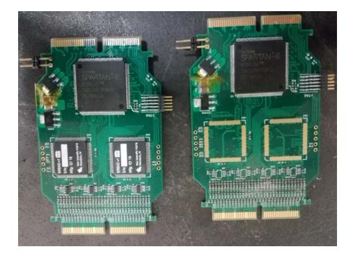
In order to apply power to the boards carefully apply 3.3 V to the right pin of the connector. This is just for the tests eventually it will be inserted to the carrier board from one end which will be connected to the PMT, while the other end will be connected to the SCROD (which will be connected via Ethernet cable with the PC) as shown in the bottom Figure on the next page.
