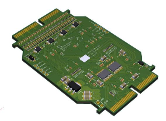
This PMT Board is basically a readout board designed for the Modular Rich (mRICH) ring imaging Cherenkov technology (RICH) which is a Key PID detectors Developed for the future electron Ion collider experiment under the eRD14 collaboration. The Position of these PMT Daughter cards in the broader system is obvious from the following Figure.
