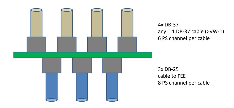
EKLM patch panel, 42 PS channels 3 required 10 PS modules (19 PS cables) required 7x DB-37 any 1:1 DB-37 cable (>VW-1) 6 PS channel per cable
