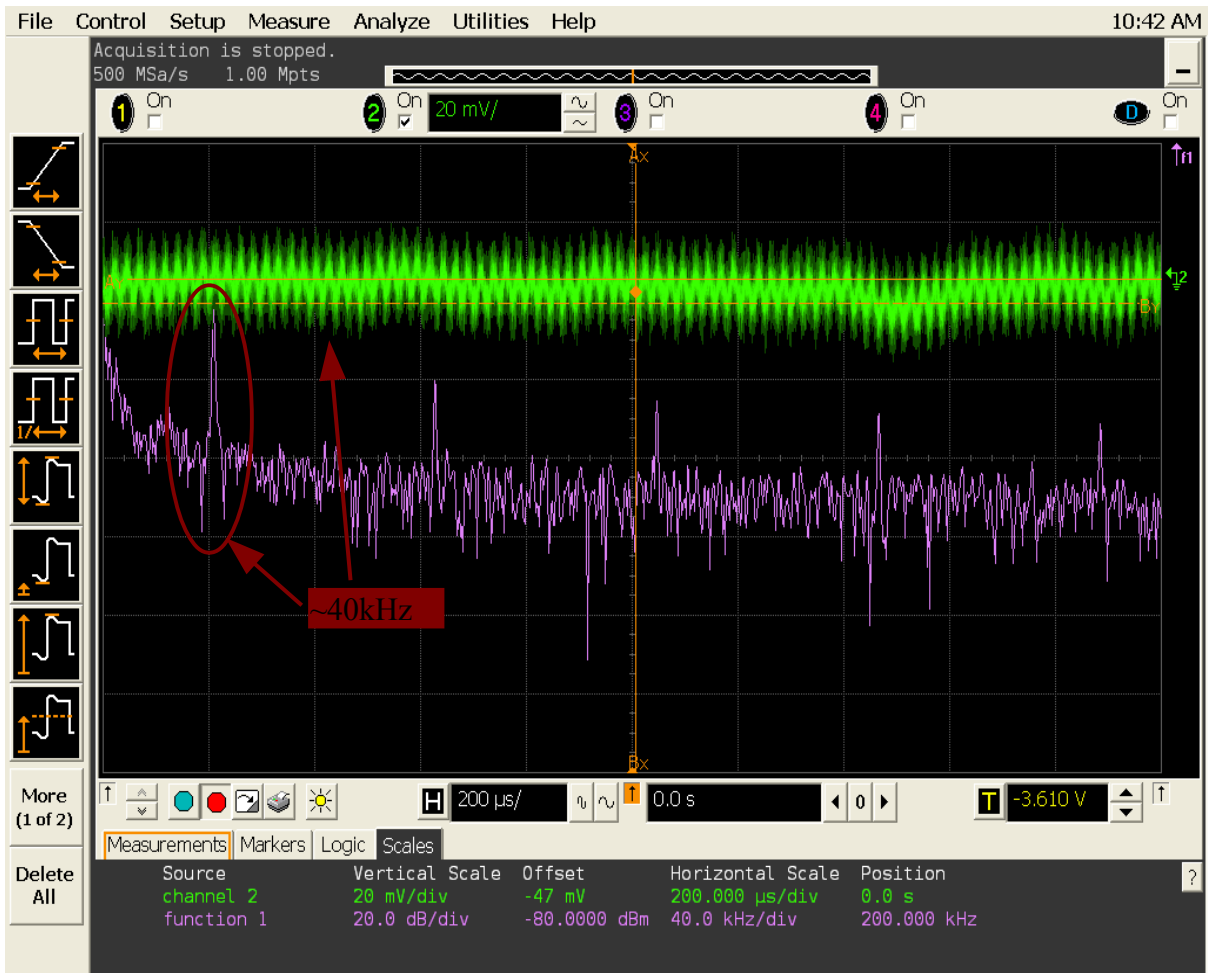
Pic-bg032702: A zoom-in look of Pic-bg032701. It's clear that the 40kHz periodic noise exists in the background.
