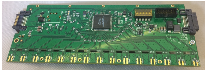
Figure 2.9: Top view of TARGETX daughtercard.
