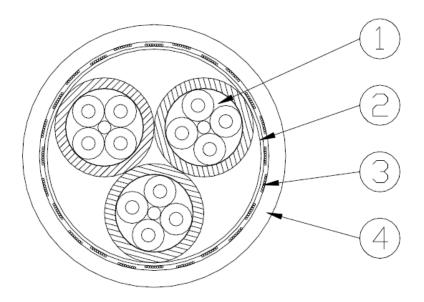
The IceRay Testbed cable is about 1.8 km in length and consists of 3 twisted-quad cables as shown above. The overall cable is also shielded and has a separate drain-wire.
