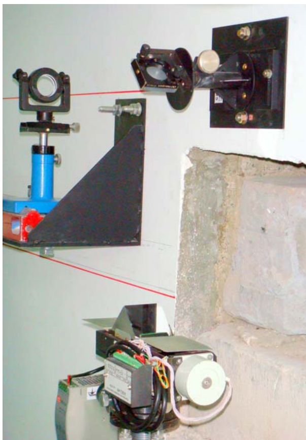
Figure 14: A closeup of the optical system, showing the second lens of the lens doublet, the 45^\circ mirror that reflects the beam vertically, and the movable prism.
