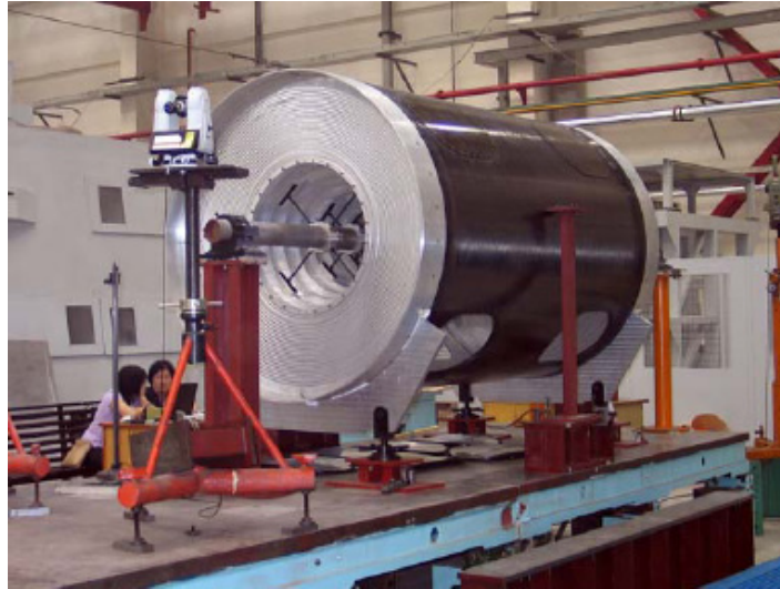
Figure 2: Completed drift chamber structure ready for shipment to IHEP for wiring - June 2005.
