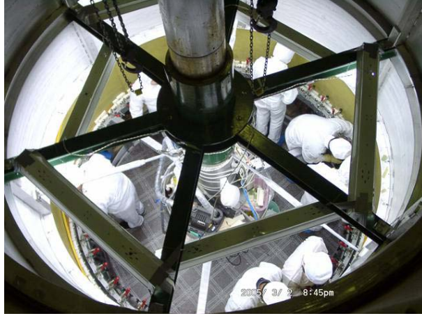
Figure 3: Winding the superconductor inside the support cylinder of the solenoidal superconducting magnet.
