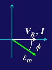
First, remember that the current phasor I is always in the same orientation as the resistor voltage phasor  $V_R$  (since the current and voltage are always in phase). From the diagram, we see that the drive phasor  $\varepsilon_m$  is *lagging* (clockwise) I. Just as  $V_C$  lags I by 90°, in an AC driven RC circuit, the drive voltage will also lag I by some angle less than 90°. The precise phase lag  $\phi$  depends on the values of R, C and  $\omega$ .
