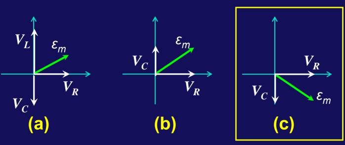
• The phasor diagram for the driven series RLC circuit always has the voltage across the capacitor lagging the current by 90°. The vector sum of the  $V_c$  and  $V_R$  phasors must equal the generator emf phasor  $\varepsilon_m$ .
