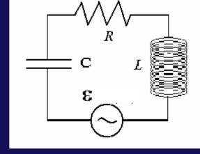
• As frequency is changed from resonance, either up or down,  $(X_L-X_C)$  no longer is zero and Z must therefore increase.
