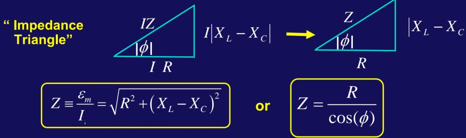
• Note that Z achieves its minimum value (R) when  $\phi = 0$ . Under this condition the maximum current flows in the circuit.
