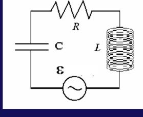
Impedance = Z = sqrt( R<sup>2</sup> + (X<sub>L</sub>-X<sub>C</sub>)<sup>2</sup>)
