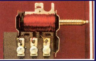
Magnet off  $\rightarrow$  plunger held in place by spring Magnet on  $\rightarrow$  plunger expelled  $\rightarrow$  strikes bell
