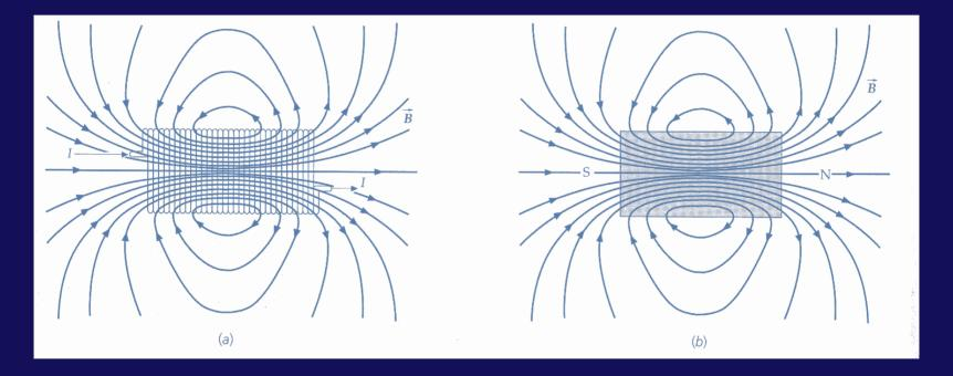
The big difference is that we can turn the solenoid on and **off**! It attracts/repels other permanent magnets; it attracts ferromagnets, etc.
