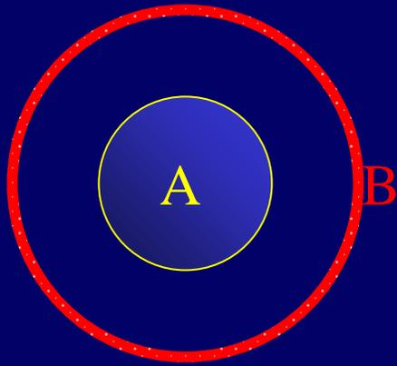
A blue sphere  $A$  is contained within a red spherical shell  $B$ . There is a charge  $Q_A$  on the blue sphere and charge  $Q_B$  on the red spherical shell.
