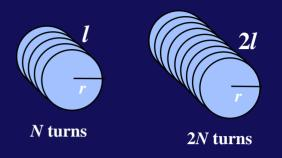
• There are twice as many turns in inductor 2; therefore the net flux through inductor 2 is twice the flux through inductor 1! Therefore,  $L_2 = 2L_1$ .
