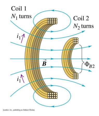
We introduce a ratio, called **mutual inductance**, of flux in coil 2 divided by the current in coil 1.
