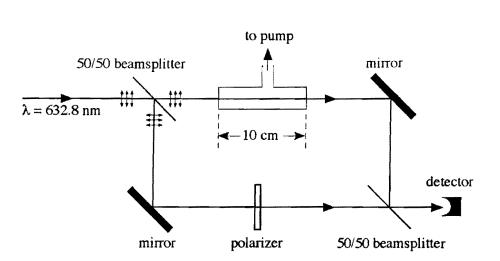
An interferometer is injected with a horizontally polarized, continuous-wave HeNe laser beam as shown in the figure above. One of the arms of the interferometer passes through a 10-cm gas cell that can be pressurized with a gas whose refractive index n varies with pressure P according to the relation n = 1+AP, where A is a constant. The other arm contains a linear polarizer. Initially, the gas cell is filled to an absolute pressure of 2.3 atm.
