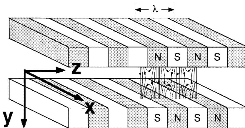
But this cannot be the *full expression* for the magnetic field in the vacuum gap at other values of y, because it does not satisfy Maxwell's equations. (There is no current  $\vec{J}$  and no time-varying  $\vec{E}$ -field on axis.)
