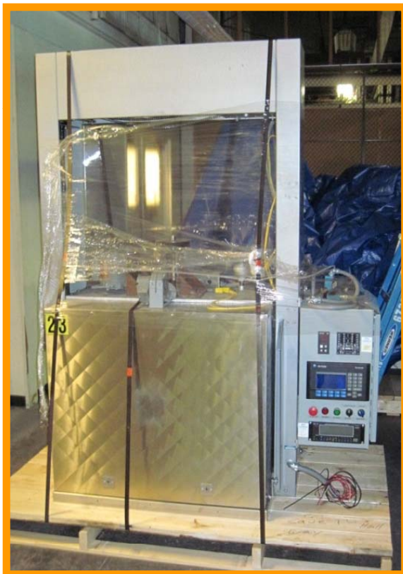
Oven and gas/vacuum control system
