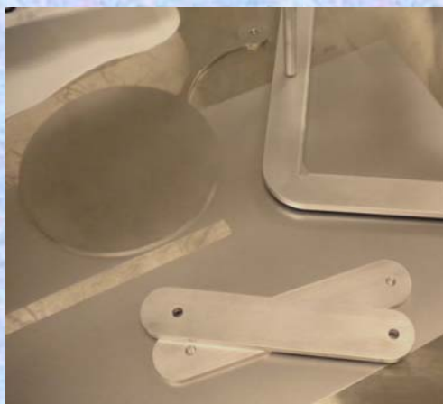
Current Bell Jar Set-Up w/ Fixturing for 33mm Sample Evaporations
