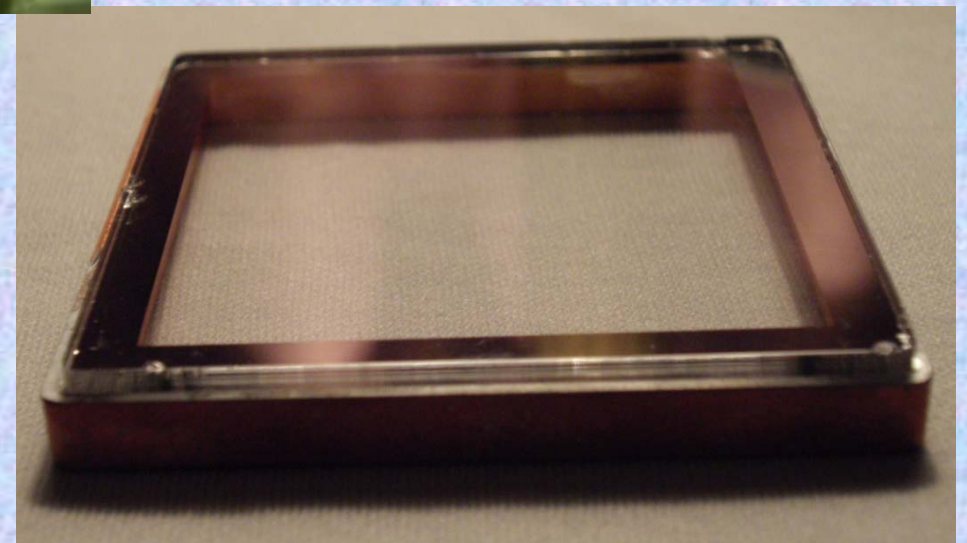
3" window test article on metal frame with Indium seal
