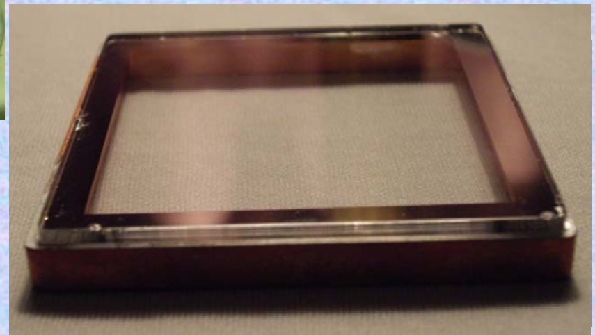
3” window test article on metal frame with Indium seal
