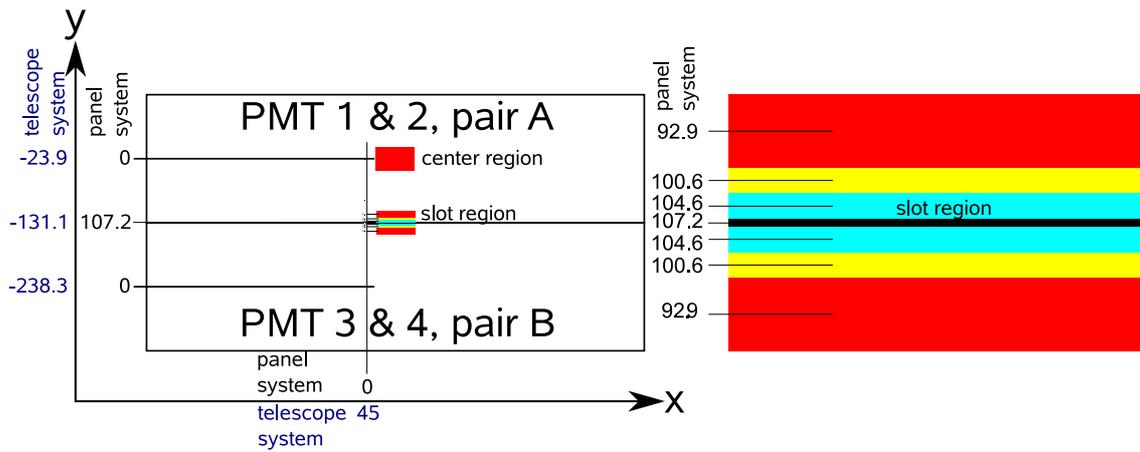
**Figure 4.62:** Coordinate systems, all values are in mm: *Left*) The two panel regions under investigation and the comparison of the beam telescope coordinate system with the panel coordinate system. *Right*) Close up of the slot region and the subdivisions.
