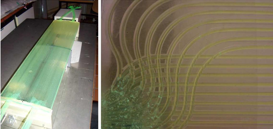
**Figure 4.29:** WLS fibers inside an ACC panel.
