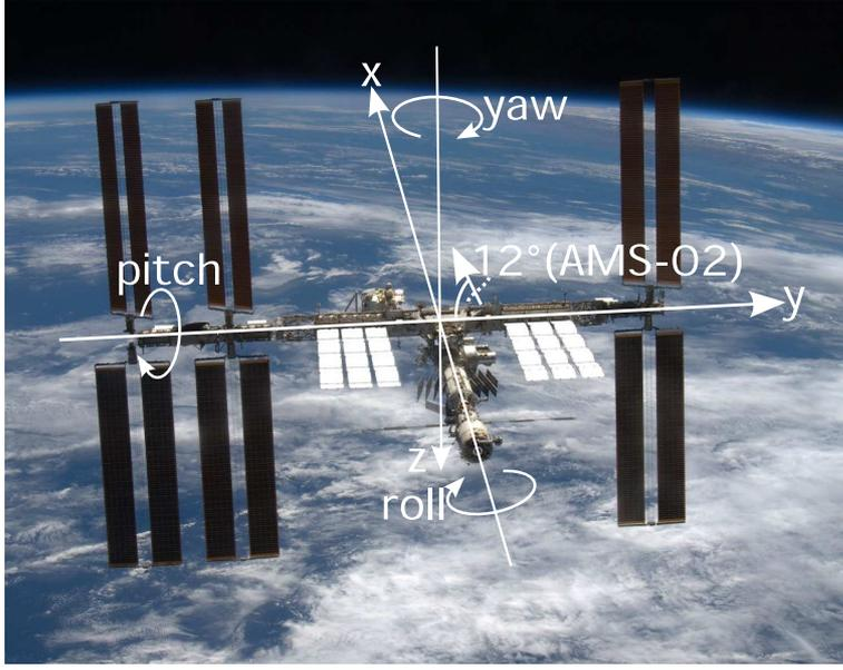
**Figure 2.19:** ISS coordinate system. Picture of the ISS taken during the NASA Space Shuttle Mission STS-126 in November 2008<sup>[82]</sup>
