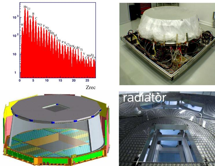
Figure 4.12: RICH detector: *Left*) Charge resolution and design. *Right*) Detector during the pre-integration and the radiator inside<sup>[112,116]</sup>.
