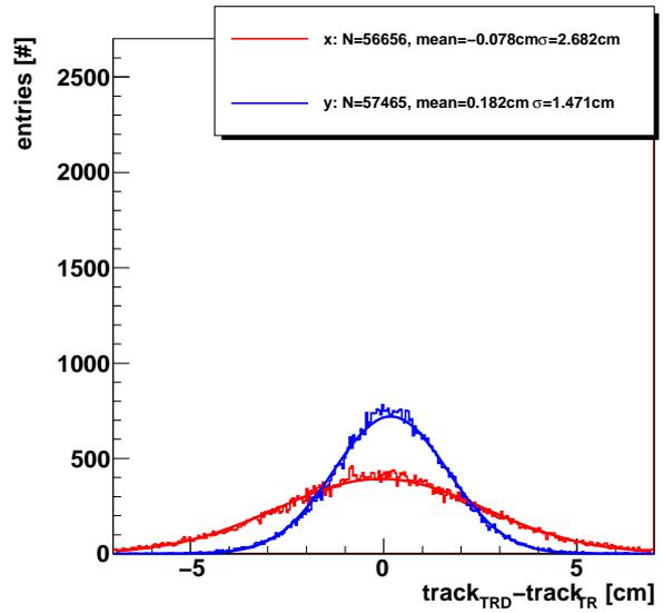
Figure 4.125:  $x, y$  projections. Distance between reconstructed tracker and TRD tracks at the  $z$  position of tracker layer 8.
