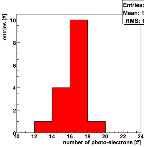
Figure 4.55: Most probable number of photo-electrons for the 16 complete ACC panels.
