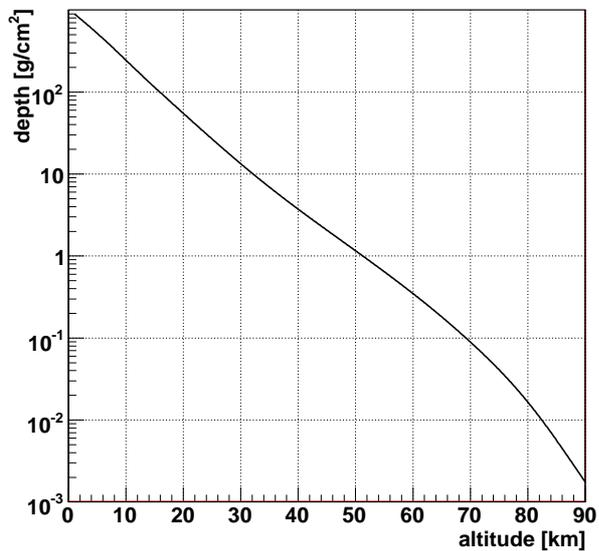
Figure 3.9: Atmospheric depth in front of the detector during summer at the South Pole as a function of altitude for tracks with  $0^\circ$  zenith angle.
