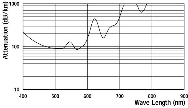
**Figure 4.44:** Attenuation length of Toray PJU-FB1000 clear fiber as a function of wavelength<sup>[127]</sup>.
