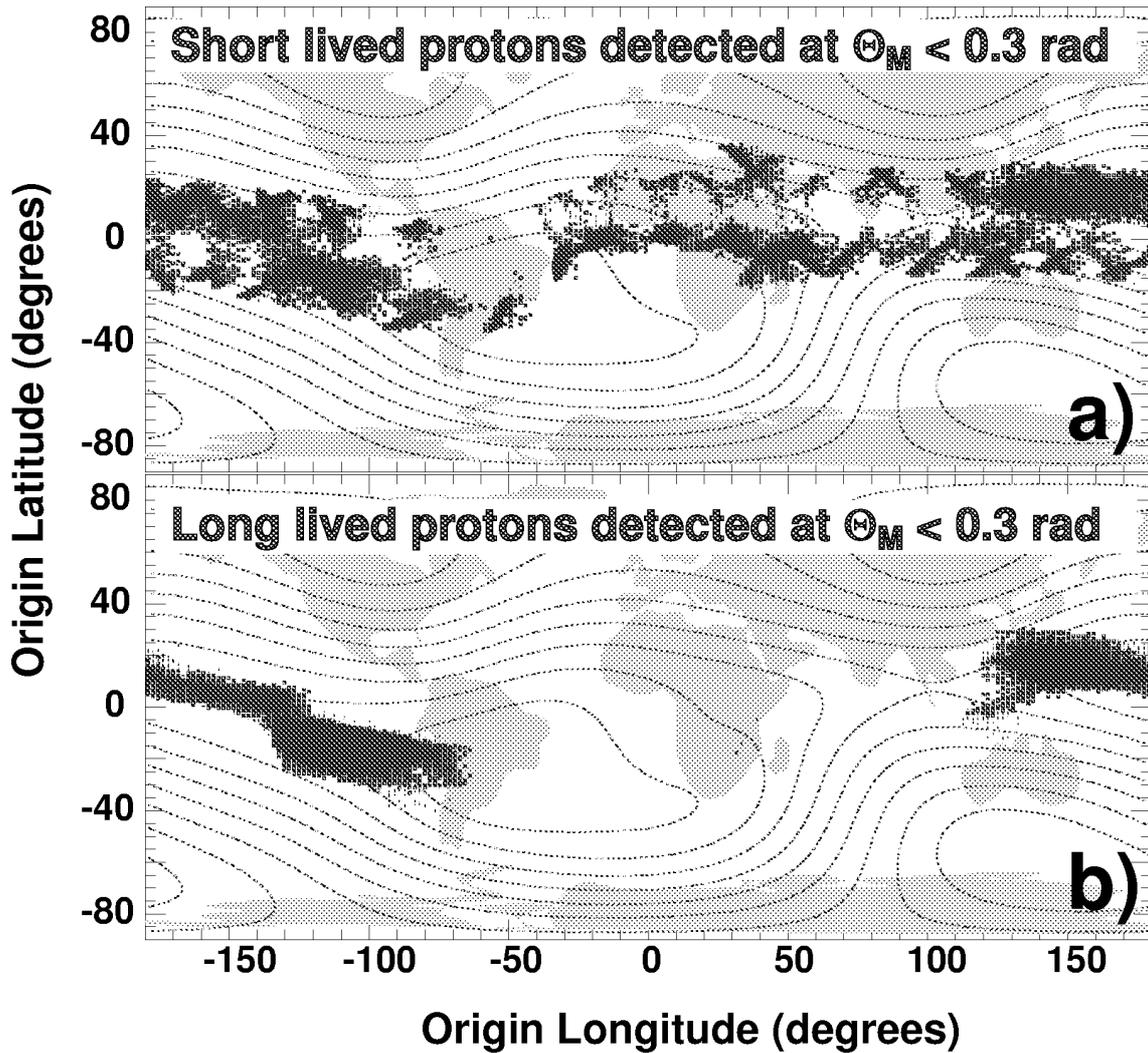
**Figure 4.3:** The geographical origin of a) short-lived ( $< 0.3\text{s}$  between detection and production) and b) long-lived ( $> 0.3\text{s}$  between detection and production) protons with  $p < 3\text{ GeV}/c$ . The dashed lines indicate the geomagnetic field contours at 380 km. Reprinted figure with permission from Elsevier<sup>[47]</sup>.
