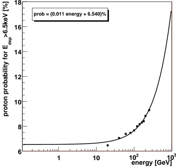
**Figure 3.34:** Probability for protons to deposit more than 6.5 keV in the proportional tubes of the TRD derived from AMS-02 TRD testbeam data<sup>[110]</sup>.
