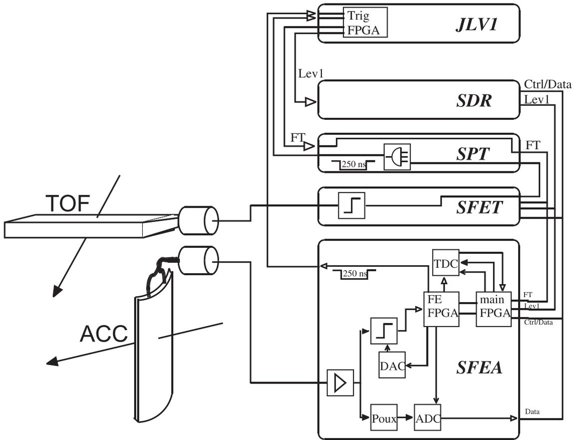
Figure 4.98: Signal processing for ACC and TOF<sup>[130]</sup>.
