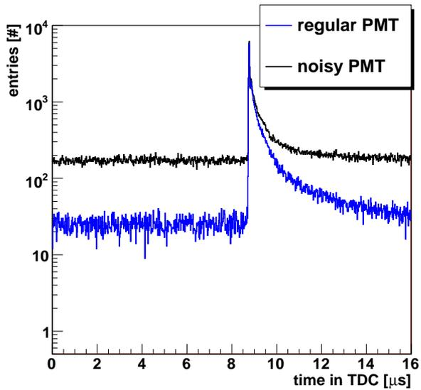
**Figure 4.121:** A regular and a noisy distribution of the TDC time stamps of PMTs connected to the SFEA2 cards in the S-crates.
