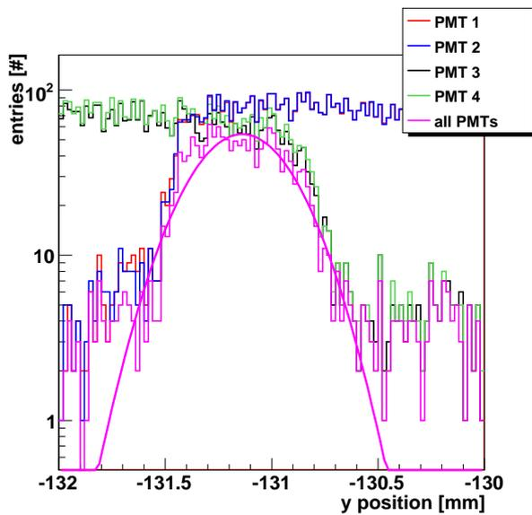
Figure 4.73: Number of events above  $3\sigma_i$  for the PMTs with respect to the  $y_{bt}$  position in beam telescope coordinates. Magenta distribution: events with all four PMTs above  $3\sigma_i$ .
