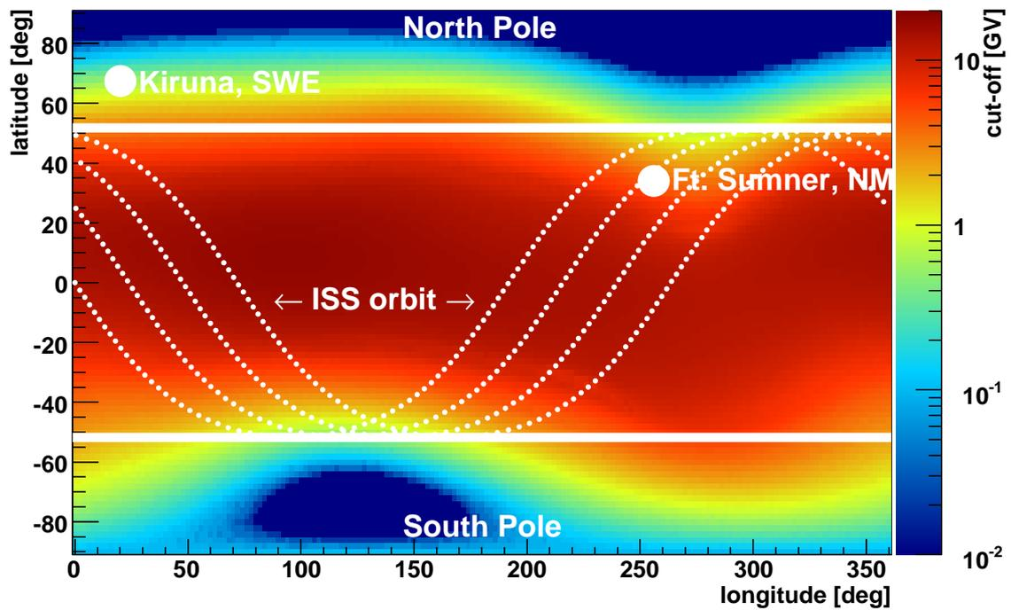
Figure 2.8: Geomagnetic cut-off at 40 km altitude for tracks with  $0^\circ$  zenith angle calculated with PLANETOCOSMICS<sup>[62]</sup>. The ISS orbit is at an altitude of about 390 km.
