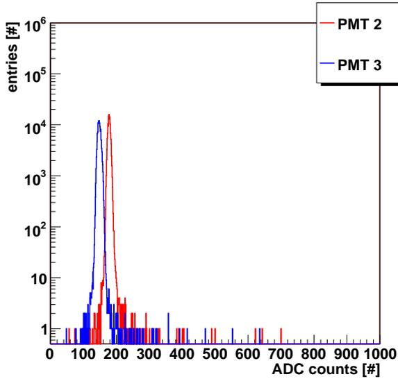
**Figure 4.106:** ADC pedestal spectra of the ACC PMTs.
