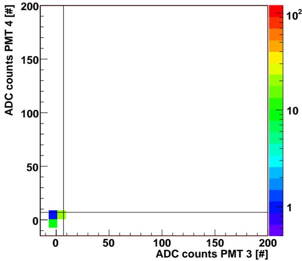
**Figure 4.75:** Pedestal corrected ADC counts of Pair B PMTs for PMT3 and PMT4  $<3\sigma_i$ . Beam telescope track points to the interval [98.6 mm,102.6 mm] in panel coordinates. The color code on the right shows the number of entries. The black lines indicate the cuts for the definition of a good event.
