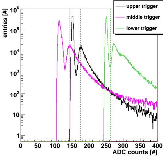
**Figure 4.104:** Data collected by the trigger counters, with cuts (dashed) used for the analysis.
