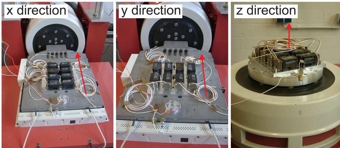
Figure 4.51: Photomultipliers mounted on the vibration table.
