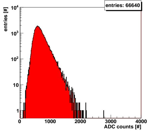
Figure 4.156: Highest ADC values normalized to the pathlength in the scintillator.
