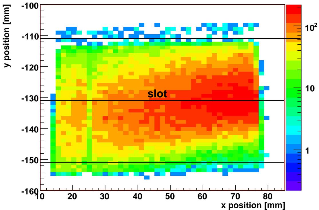
**Figure 4.63:** Beam profile collected with the telescope and defined by the large trigger counters. The lines indicate the  $y_{bt}$  range of hits used in the analysis. The color code on the right shows the number of entries.
