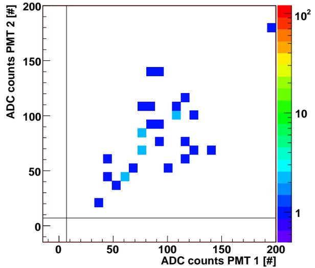
**Figure 4.76:** Pedestal corrected ADC counts of Pair A PMTs for PMT3 and PMT4  $<3\sigma_i$ . Beam telescope track points to the interval [98.6 mm,102.6 mm] in panel coordinates. The color code on the right shows the number of entries. The black lines indicate the cuts for the definition of a good event.
