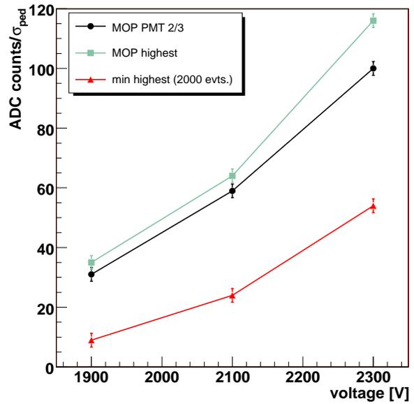
Figure 4.89: MOP and minimum normalized ADC values at different voltages. The normalized MOP values for PMT 2 and 3 are very close so that the mean value is shown. The curve labeled 'highest' depicts the highest of the two PMT values for each event.
