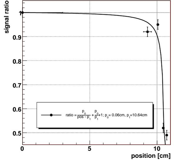
**Figure 4.93:** Behavior of one PMT MOP value across the panel from the testbeam measurements normalized to the center of the panel at 0 cm. The slot position between two panels shows a signal drop by about 50 %.
