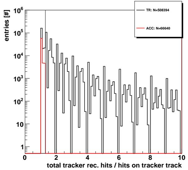
**Figure 4.140:** Ratio of reconstructed tracker hits to tracker hits on the fitted track. The black distribution shows the ratio values for tracker tracks pointing to the ACC matching the run, TOF, TRD and tracker cuts in Tab. 4.9 but not the tracker noise requirement. The red ratio distribution shows the values of events selected for the ACC analysis matching all requirements in Tab. 4.9. The vertical line indicates the cut for the event selection.
