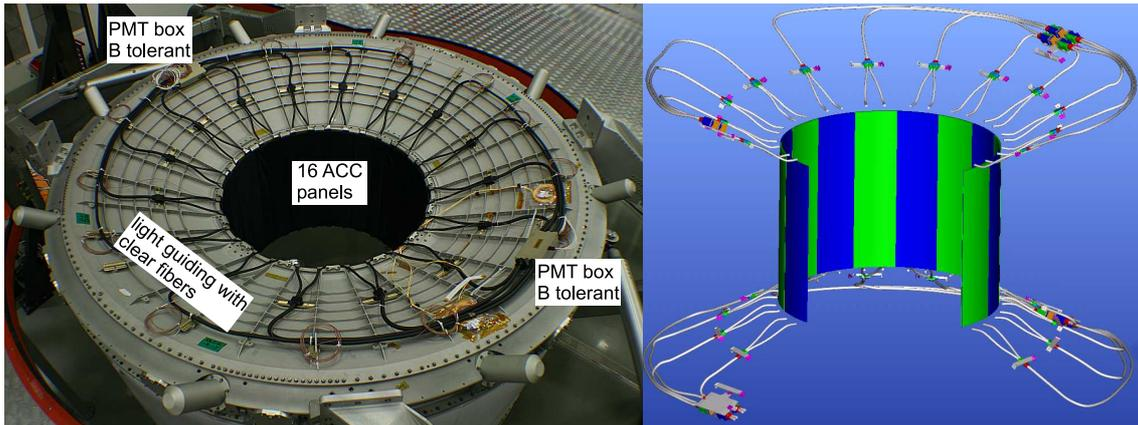
Figure 4.23: The AMS-02 anticoincidence counter system surrounds the silicon tracker.
