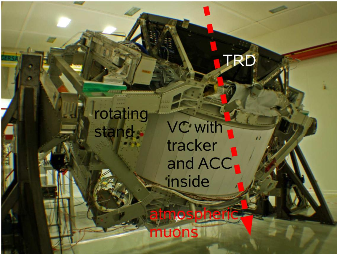
**Figure 4.118:** AMS-02 taking atmospheric muon data after the pre-integration. VC denotes the vacuum case for the helium tank.
