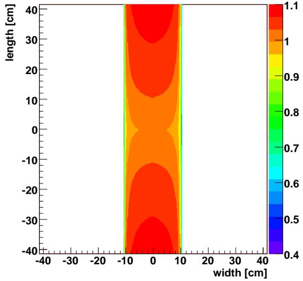
**Figure 4.95:** Expected MOP value behavior for the highest ADC value with PMTs on both ends of the panel. The color code on the right indicates the relative signal change.
