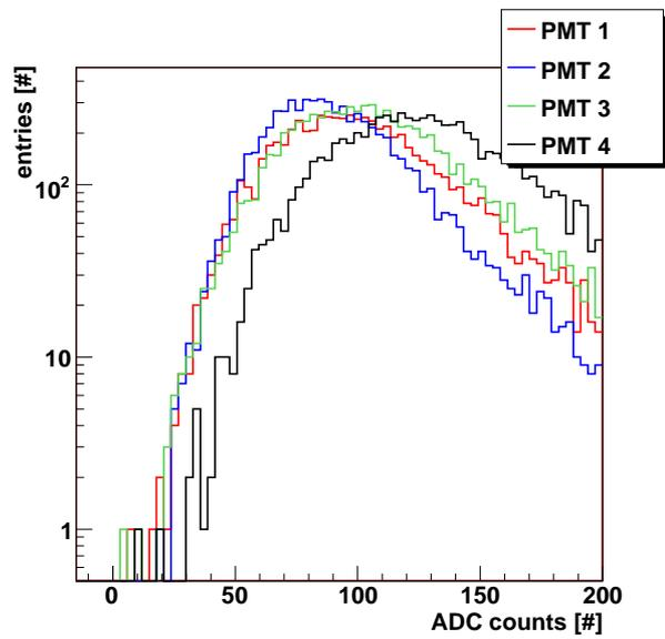
Figure 4.67: Pedestal corrected ADC spectra for all PMTs at position  $y_p = 92.9$  mm in panel coordinates.
