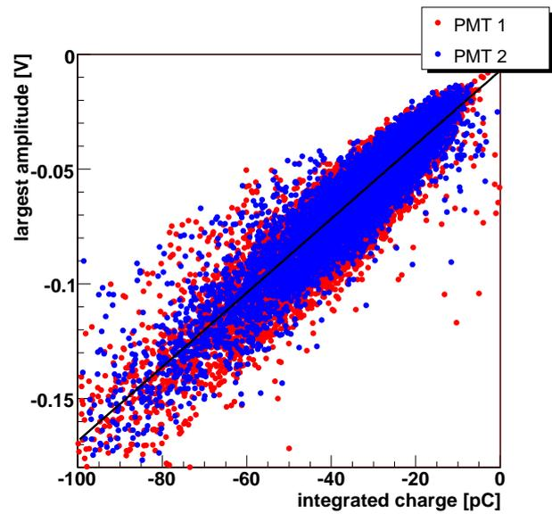
Figure 4.72: Correlation between largest amplitude and integrated charge.
