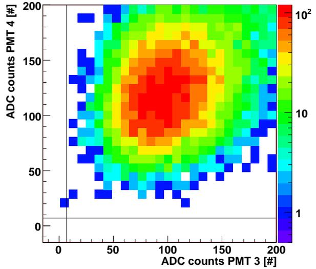
**Figure 4.78:** Pedestal corrected ADC counts of Pair B for clean single tracks. Beam telescope track points to the interval [98.6 mm,102.6 mm] in panel coordinates. The color code on the right shows the number of entries. The black lines indicate the cuts for the definition of a good event.
