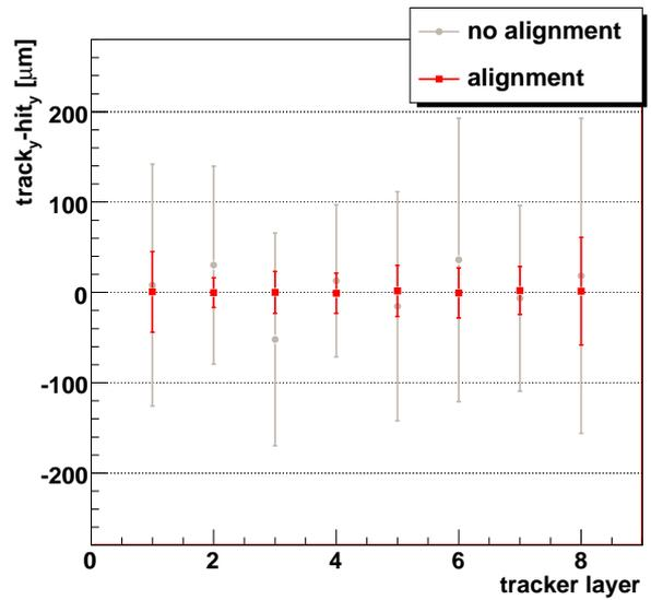
Figure 4.127: Mean tracker residuals in  $y$  direction before and after alignment with RMS as error bars.
