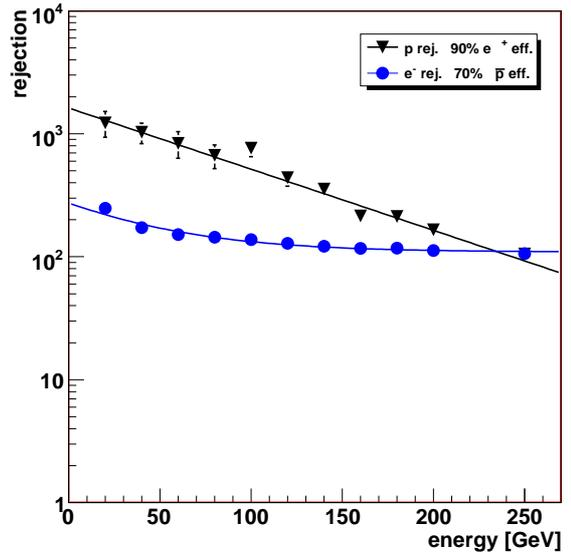
**Figure 4.170:** Proton and electron rejection factors in the TRD<sup>[110]</sup>.
