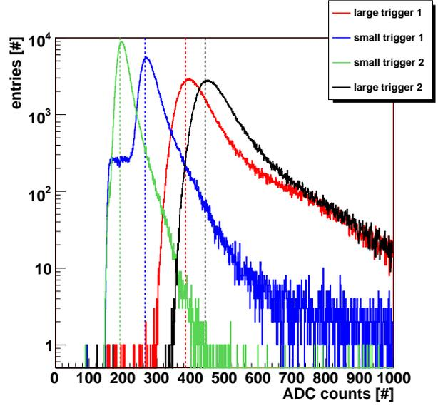
**Figure 4.65:** Trigger spectra for large and small counters. Cuts (dashed lines) are at 385, 265, 191 and 443 ADC counts.
