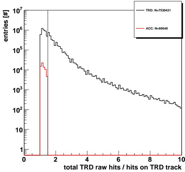
**Figure 4.139:** Ratio of raw TRD hits to hits on TRD track. The black distribution shows the ratio values for TRD tracks pointing to the ACC matching the run, TOF and TRD cuts in Tab. 4.9 but not the TRD noise requirement. The red ratio distribution shows the values of events selected for the ACC analysis matching all requirements in Tab. 4.9. The vertical line indicates the cut for the event selection.
