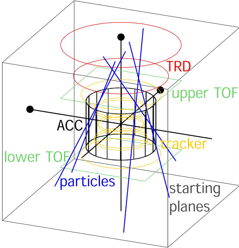
**Figure 4.145:** Model for simple AMS-02 simulations of flux, acceptance and pathlength in the scintillator material of the ACC. Calculations are made without magnetic field. The gray box indicates the starting planes for the simulation and the black lines the ACC cylinder. The blue lines illustrate particles hitting the TRD (red), the upper TOF (green), at least 3 tracker layers (orange) and the ACC.
