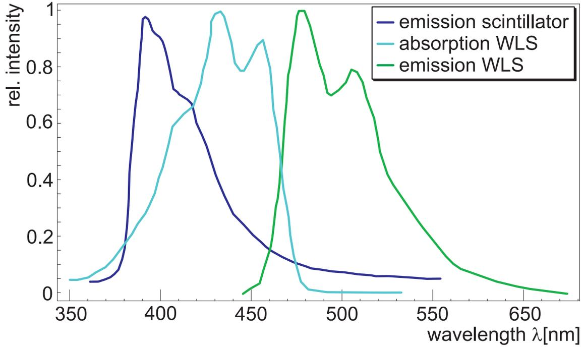
**Figure 4.35:** Emission and absorption spectra of the scintillator material and the wavelength shifting fibers<sup>[120,121]</sup>.
