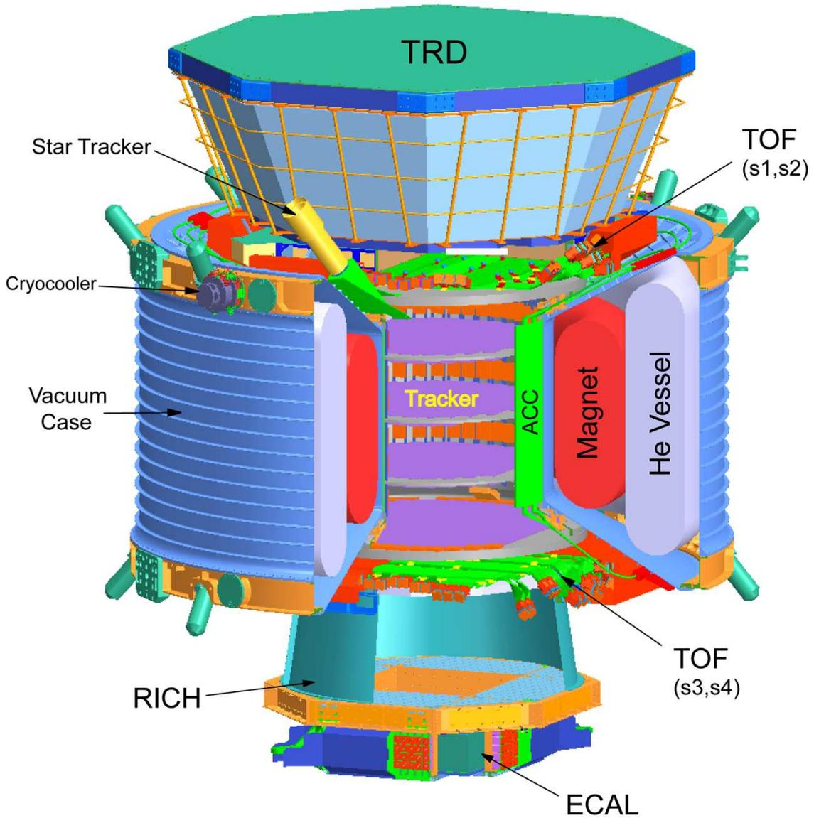
Figure 4.4: The AMS-02 experiment<sup>[112]</sup>.
