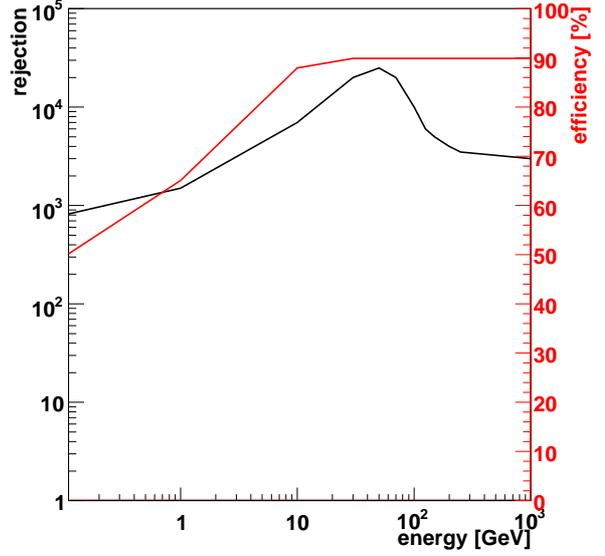
**Figure 3.35:** Electron (proton) rejection (black) and antiproton (positron) efficiency (red) of the electromagnetic calorimeter vs. the reconstructed momentum<sup>[61]</sup>.
