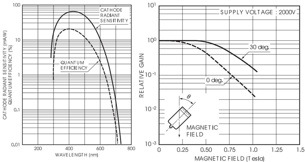
**Figure 4.49:** *Left)* PMT quantum efficiency vs. wavelength. *Right)* Change of PMT gain in magnetic field<sup>[119]</sup>.
