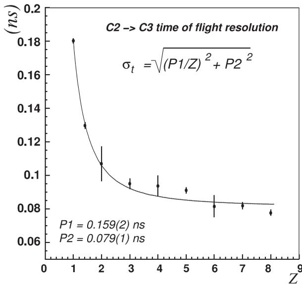
Figure 4.8: TOF: time resolution vs. charge<sup>[114]</sup>.
