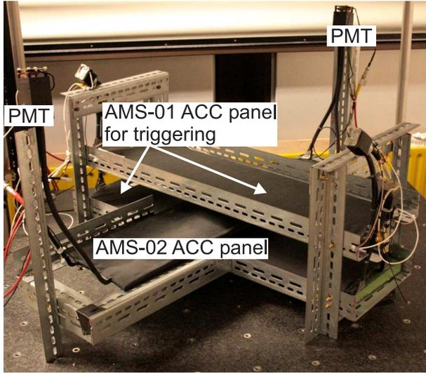
**Figure 4.30:** Test setup for the qualification of the scintillator panels and the photomultiplier tubes.
