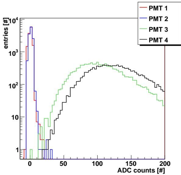
**Figure 4.77:** Pedestal corrected ADC counts for all ACC PMTs. Beam telescope track points to the interval [98.6 mm,102.6 mm] in panel coordinates.
