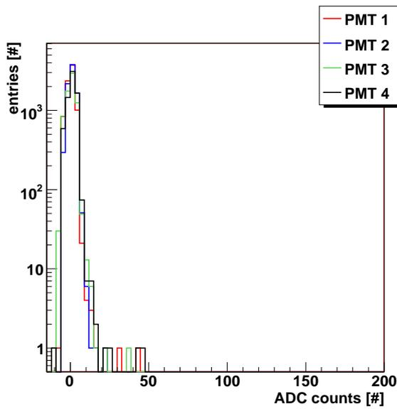
Figure 4.66: Pedestal measurements for all PMTs.
