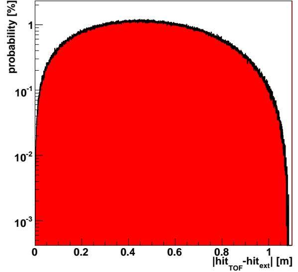
**Figure 4.168:** Probability for the distance between external events and TOF events in the tracker normalized to the number of TOF triggers.
