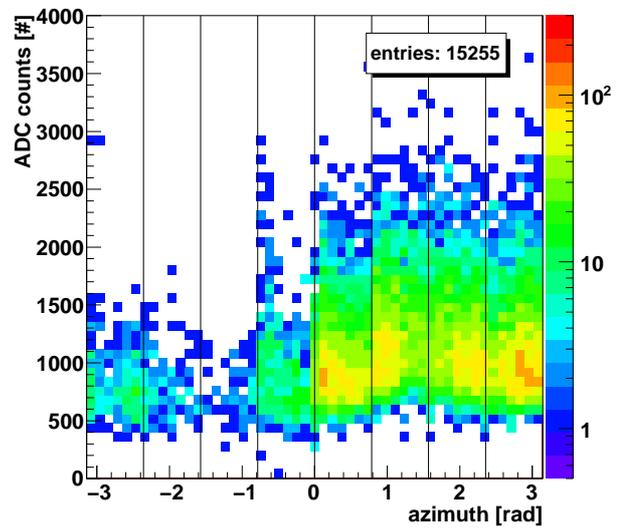
Figure 4.152: ADC values of the  $+z$  PMTs as a function of the azimuthal angle for the case that these PMTs have recorded the highest ADC value. The vertical lines indicate the slots between the ACC sectors. The color code on the right shows the number of entries.
