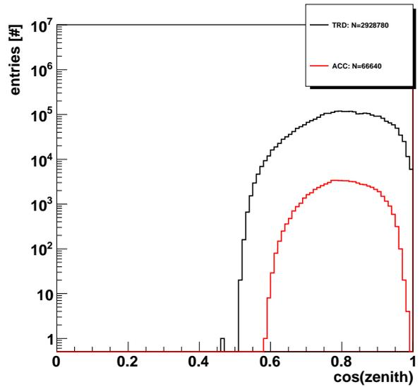
Figure 4.142: Zenith angle distributions on the ACC using only TRD tracks and for new tracks in the tracker surviving all cuts.
