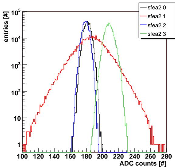
Figure 4.114: ADC spectra of the SFEA2 board of the qualification S-crate during temperature variations in the range between  $-20^{\circ}\text{C}$  and  $60^{\circ}\text{C}$ . A test pulse was injected in channel 1 only.
