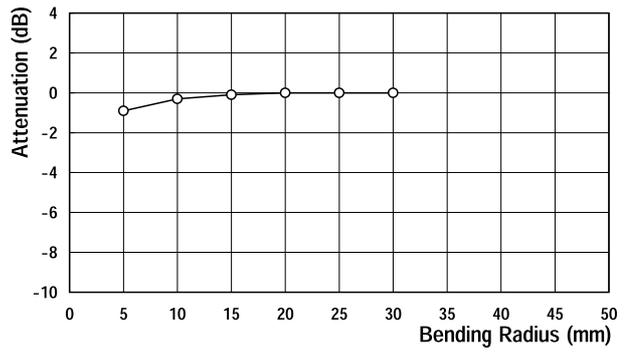
**Figure 4.45:** Bending loss of Toray PJU-FB1000 clear fiber as a function of radius<sup>[127]</sup>.
