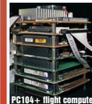
The **flight computer is the central computing unit** for receiving **commands** and sending **data** during flight from/to ground as well as for the **rotation calculation** of the gondola. The gondola communication is handled by Ethernet communication and the ground communication via serial lines. For an efficient way of handling the various tasks a multi-threaded approach was chosen.
