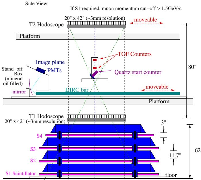
Figure 3: Schematic drawing of the FDIRC prototype located in a large cosmic ray telescope built at SLAC.
