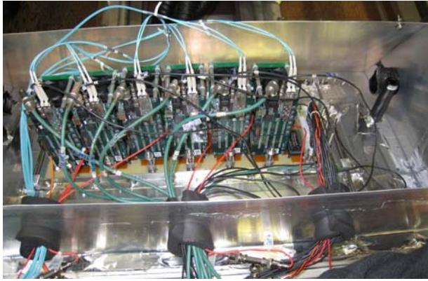
Figure 4: Integrated readout of six H8500 64-anode PMTs (384 channels). LC-Duplex fibers transport the data and are less bulky than the green RG-58 cables used for power.
