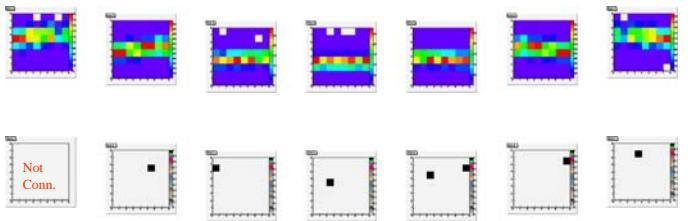
Figure 5: Comparison of results between Geant4 MC (top), where the color corresponds to the intensity of photons observed in each pad, and typical single cosmic data event (bottom), where each black square corresponds to a single recorded Cherenkov photon.
