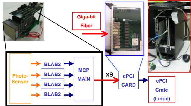
Figure 2: Components of the waveform sampling readout of the Focusing DIRC prototype. BLAB2 digitizer ASICs are placed immediately behind the 64-anode phototube and digitized events are carried over Giga-bit fiber links to a cPCI-based data acquisition system.
