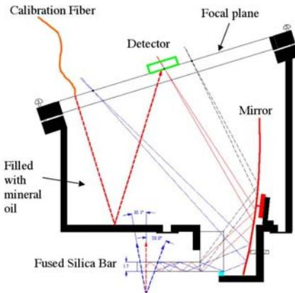
Figure 1: Principle of the Focusing DIRC prototype [3-7], where the angular error contribution due the finite bar thickness is removed by focusing parallel rays onto the same image plane location.
