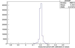
(Left) Measured period after calibration from last time indicated an overall scale offset. Measured 4.2 ns but expected 4.17 ns.
