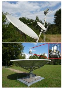
All antennas vertically oriented, with linear polarized receivers.
