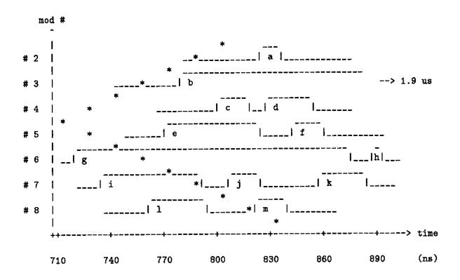
Figure 1: timing chart of "the event". \* shows timing diagram for a muon track perpendicular to the string and crossing the string between modules # 4 and 5, as an example.
