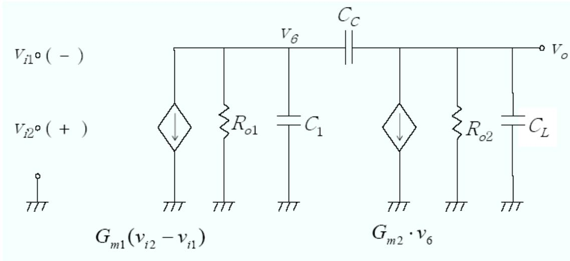
KCL at  $v_6$  and  $v_o$  nodes
